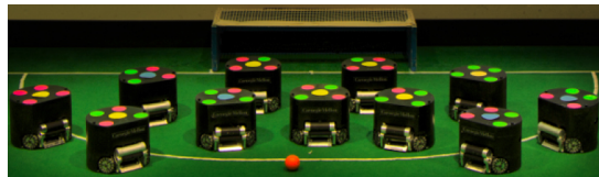
Figure 1: All the CMDragons 2015 robots (6 play at a time), champions of the RoboCup Small Size League of robot soccer. ( Hardware designed and built by Mike Licitra, and carefully maintained by Joydeep Biswas and Richard Wang. )
